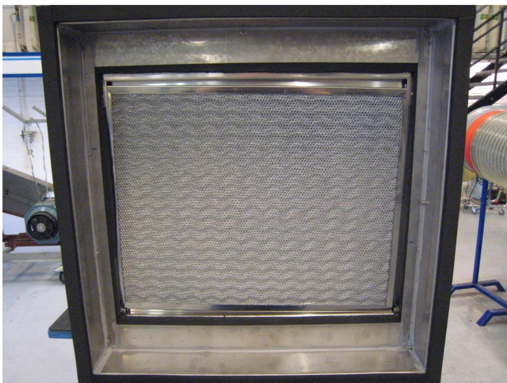
Fig 6. Three FE600 mounted in series in the duct section, front side
